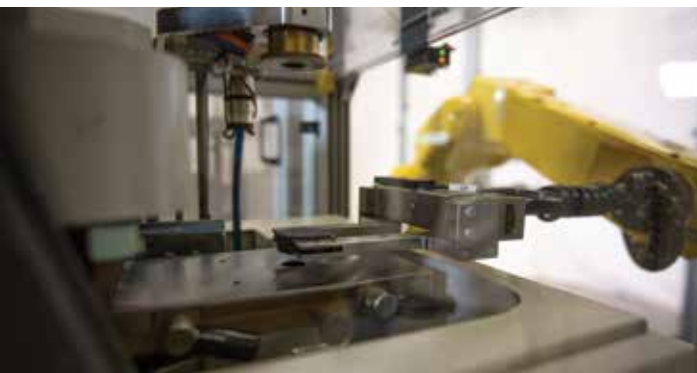
ARL iSpark robot access for automatic analysis
