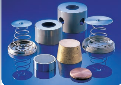
Small and large cassettes can accommodate samples of various sizes
