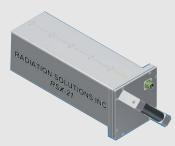
The **RS-725/21** system is a 3"x3" (21 cu ins) Sodium-lodide detector mounted in a square housing. Normally the face of the detector is mounted as close as possible (4-6") from the measurement point and installed in a 1" steel collimator during installation. This collimator reduces local
