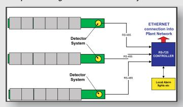
The RS-725 Controller is connected directly to the Plant Network via the Ethernet port giving the RSO direct access to alarm data.
