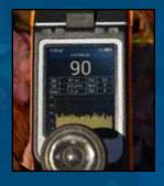
The SR-10 Super-RIID has a large color display featuring an automatic "black and white" high contrast mode for superior visibility in high sunlight operation.
