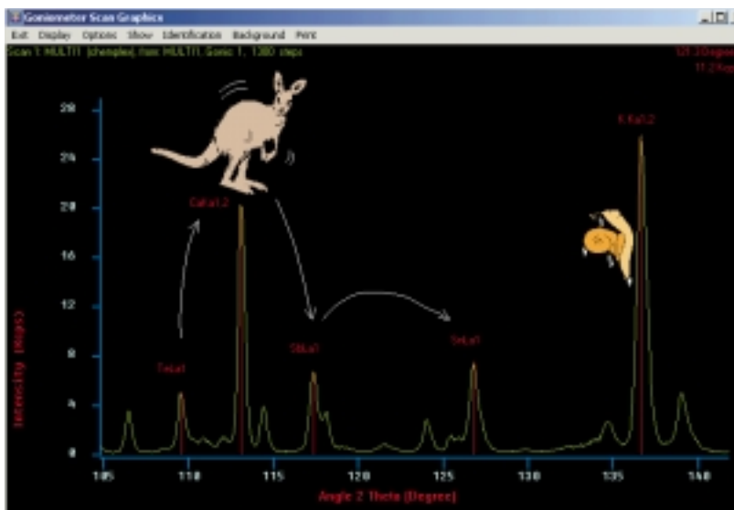
Either peak to peak hopping or scanning can be used for standardless analysis
